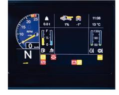
Multifunctional service and maintenance display makes it easy to check transmission oil level, plus hydraulic and electronic components.
