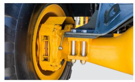
The booster pump delivers a higher augmented-thrust ratio, more stable braking performance, and more convenient daily maintenance thanks to its being mounted on the body's side.
